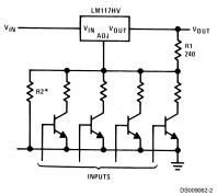
5V Logic Regulator with Electronic Shutdown\*
