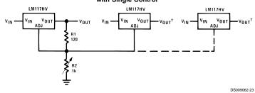
\*All outputs within ±100 mV †Minimum load — 10 mA
