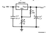
Full output current not available at high input-output voltages
