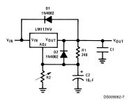
FIGURE 3. Regulator with Protection Diodes
